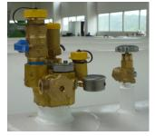
Multivalve REGO or OMECA combines double back check filler valve, vapour equalizing valve with excess flow, pressure relief valve, service shut-off valve, Junior level gauge and pressure gauge. Additionally installed is liquid service valve.
