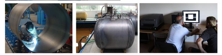
Our commitment to the quality is supported by the fact that we manufacture in a brand new plant on modern machinery, our staff is good trained and long experienced in the field of LPG. Our tanks are manufactured according to AD Merkblatt 2000 and certified according to the European Pressure Equipment Directive 2014/68/EU (modules B+D, HP 0, outside coating according to DIN 4681-3).
