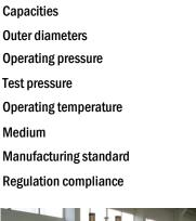
500 - 125 000 liters Standard D 1250 / 2000 mm. Other diameters on enquiry 15,6 bar (other pressures possible) min. 22,3 bar Standard -20/+40 °C (other temperatures possible) Liquefied gas DIN 51622 / EN 589 AD-Merkblatt 2000 European Pressure Equipment Directive 2014/68/EU, modules B/G + D
