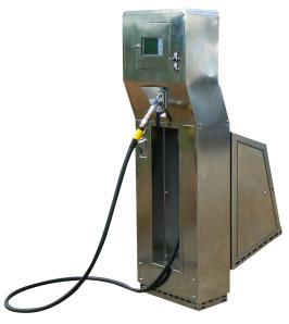
Specially developed design for use on autogas filling units. The key element of the dispenser is a mass flow meter with its own temperature compensation, which exactly measures dispensed amount on the principle of Coriolis force. Data from the flow meter is then processed by measuring unit, which transmits it to the fuel station terminal.
