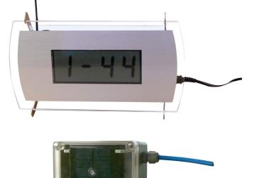
**TRANSMITTER-RECEIVER KRT01** is used to extend the range or to transmit data under difficult conditions. The device does not require any operating or maintenance. The device is powered by solar cell.
