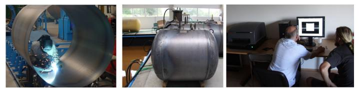
Our commitment to the quality is supported by the fact that we manufacture in a brand new plant on modern machinery, our staff is good trained and long experienced in the field of LPG. Our tanks are manufactured according to AD Merkblatt 2000 and certified according to the European Pressure Equipment Directive 97/23/EC (modules B+D, HP 0, outside coating according to DIN 4681-3).
