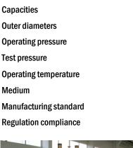
500 - 100 000 liters Standard D 1250 / 1600 / 2000 mm. Other: 800 / 1000 / 2500 mm 15,6 bar (other pressures possible) 25 bar -20/+40 °C or -40/+40 °C Liquefied gas DIN 51622 / EN 589 AD-Merkblatt 2000 European Pressure Equipment Directive 97/23/EC, modules B/G + D
